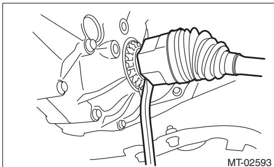
9) Remove the differential side retainer oil seal.
