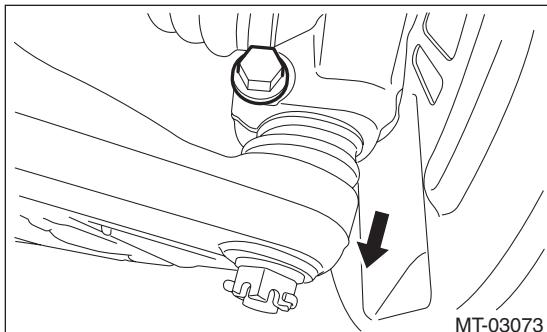
8) Using a crowbar, separate the left and right front drive shafts.
